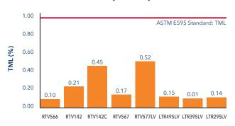
$<sup>^{\</sup>star}\text{Low outgas testing performed using ASTM E595 Low Outgas Test Procedures in a vacuum environment.} Test results. Actual results may vary. \\$
